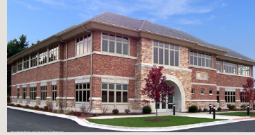
This example shows an office building with a primary facade using brick with stone as an accent material, meeting desired natural color palette.
