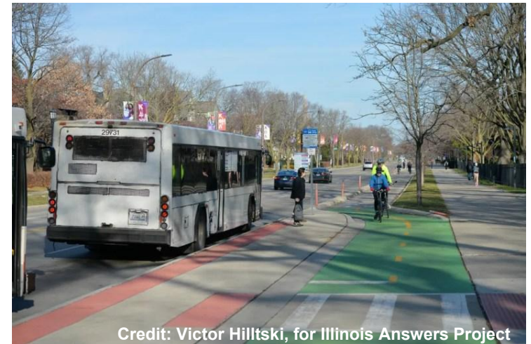
Figure 7: Adding protected bike lanes on Sheridan Road in Evanston resulted in lower motor vehicle speeds
